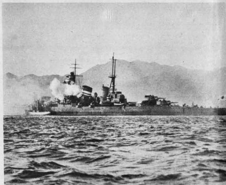
Nachi Class , with Atagos and Mogamis, are Japan's biggest and most heavily armed cruisers. Battery arrangement is same as on the Atagos (2-1-A-2), but vertical bridge structure is more simplified (see cover).
